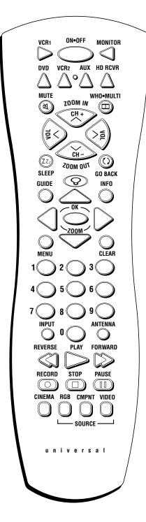
**ON•OFF** Toggles power on and of for the components that you have programmed. For example, if you are in VCR mode, turns VCR on and off.
